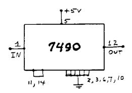
The divide by 10 configuration is shown in the schematic at left. Check the table below for other dividers.
