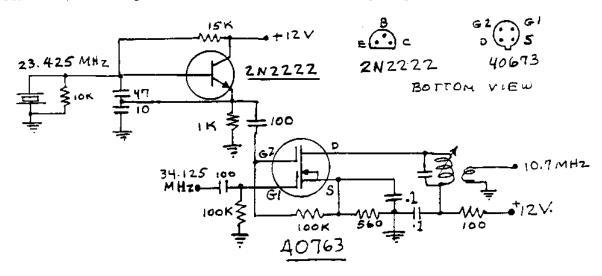
2N2222 is an all purpose NPN transistor, rated at of .625 watts, at frequencies up to 300 MHz.
