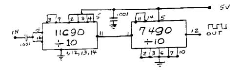
A simple two chip frequency divider that can be used to divide signals by 100. By changing connections on the 7490, you can also divide by 50, 60, 70, 80 or 90.
